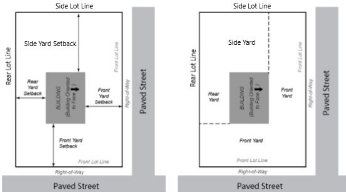
Figure 4: Typical lot lines and setback locations for a corner lot with the building oriented toward the wider street frontage (left image) and typical yard locations (right image).
