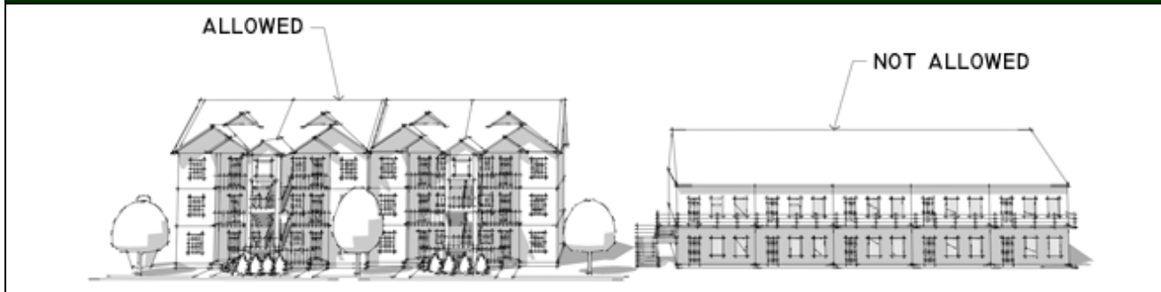
Figure 5.1.203 Illustrative Application of Building Design Standards
